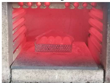
Fig 2. PWHT of steel P91 for 2h
