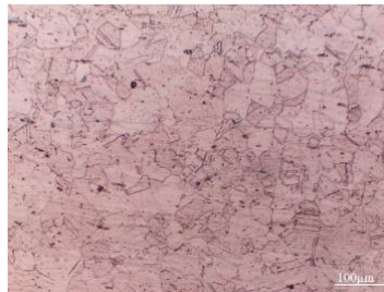
Figure 9 Microstructure of base material 12X18H12T
