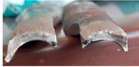
Figure 5 Fracture of specimen 1
