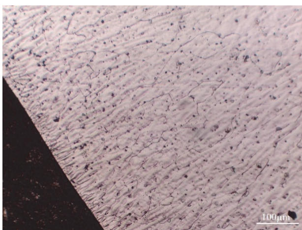
Figure 10 Microstructure of buttering layer of X10CrMoVNb9-1
