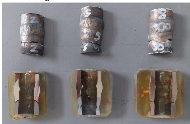
Fig 6. Fracture in HAZ of P91 as result of overheating during buttering with Thermanit Nicro 82
