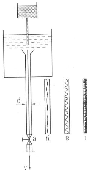
Fig. 6.16: Scheme of the Reynolds experiment
