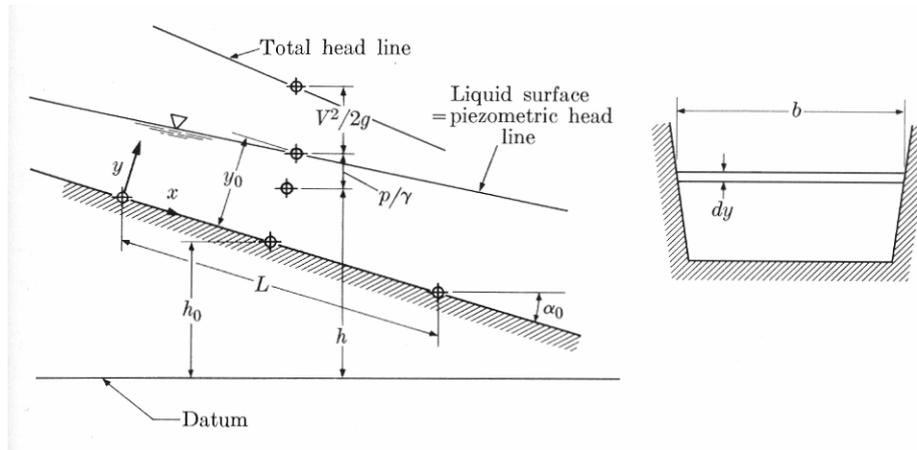
Fig. 8.17: Notations for one-dimensional open channels
