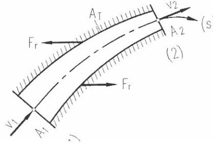
Fig. 5.4: Stream tube with solid boundaries
