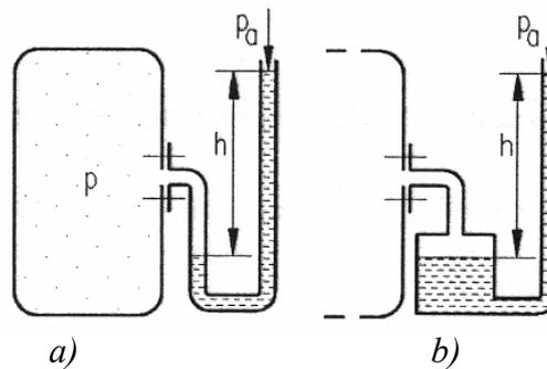
Fig. 2.8: Hydrostatic manometer; a) U-tube and b) Vessel manometer
