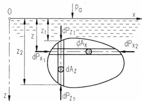
Fig. 2.23: Acting forces on an immersed body
