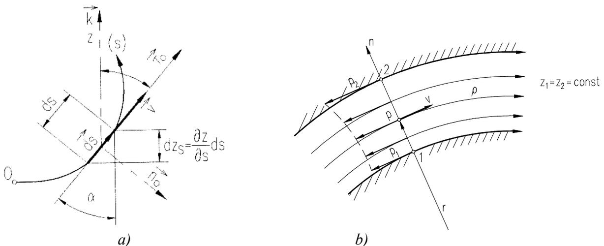
Fig. 4.1: One dimensional gravity flow
