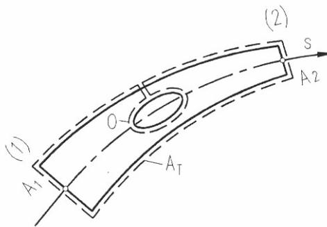
Fig. 5.2: Bounding surfaces of a stream tube
