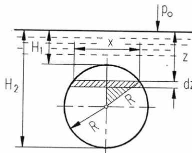
Fig. 5.11: Discharge into the atmosphere through circular opening
