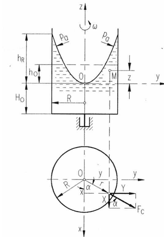
Fig. 2.13: Rotation of a liquid container around vertical axis
