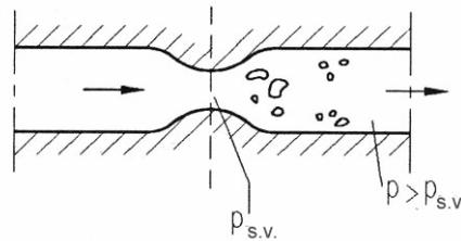
Fig. 5.17: Generation of cavitation in non-rotational channel
