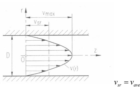
Fig. 6-7: Steady laminar flow in a circular tube of a constant diameter
