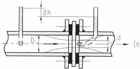
Fig. 5.6: Concept of an orifice meter co
