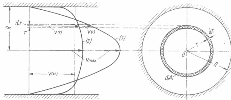
Fig. 8.2: *Velocity distribution in a pipe cross-section*
