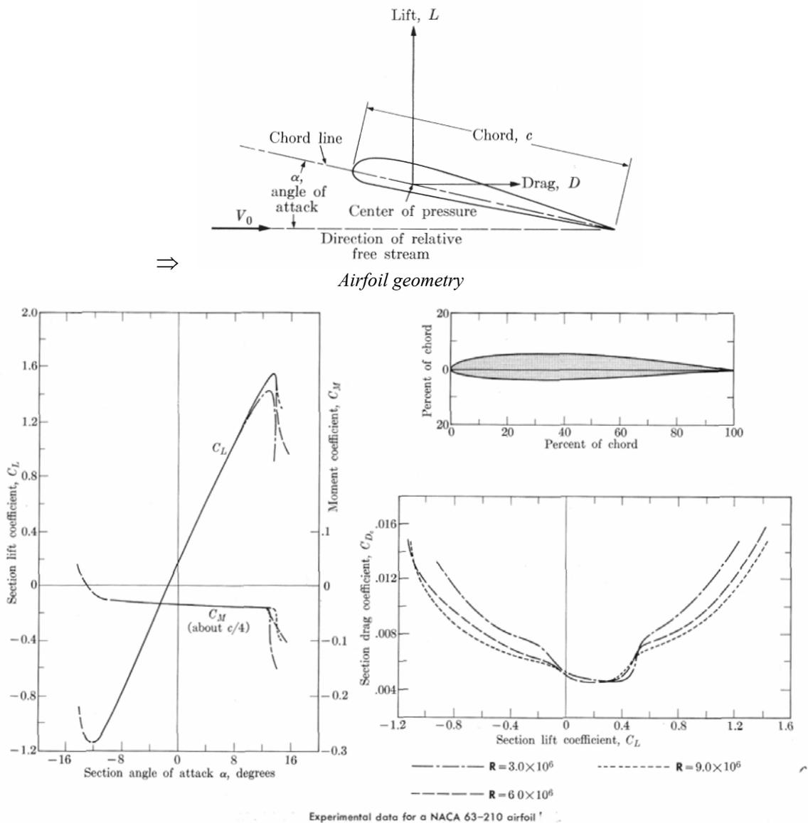
Fig. 8.20: Experimental data for the lift and drag coefficients for an airfoil
