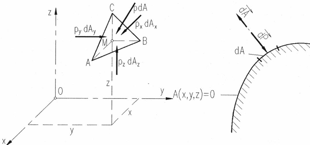
Fig. 2.1: Equilibrium of surface forces on a infinitesimal fluid element
