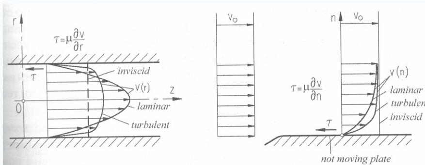
Fig. 6.1: The influence of the shear stress for viscous fluid flow
