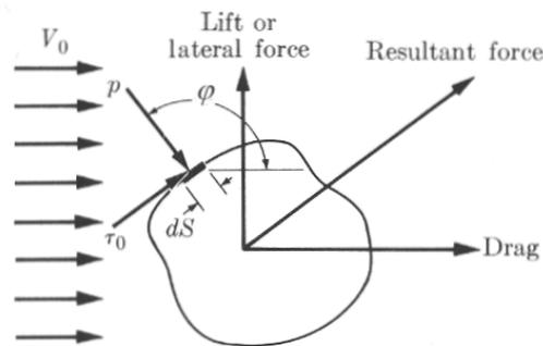
Fig. 6.12: Definition diagram for flow-induced forces
