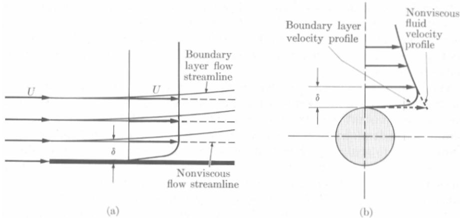
Fig. 6.10 a,b: Boundary layer versus slip flow: (a) flat plate ;(b) cylinder
