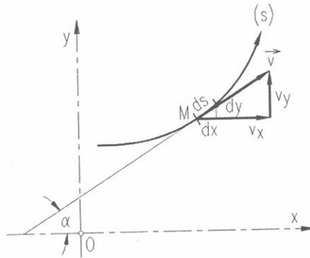
Fig. 3.5: Slope of a streamline
