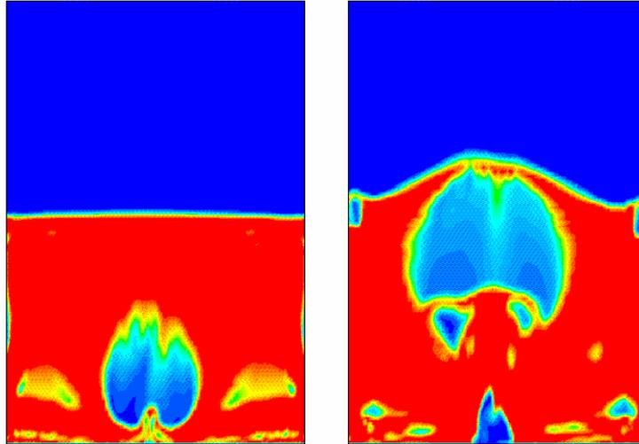
An initially stationary bed of solids is fluidized by the action of a central jet. Red indicates regions of maximum solids volume fraction ( $\sim 0.6$ ), and blue indicates regions of maximum air volume fraction (1.0).
