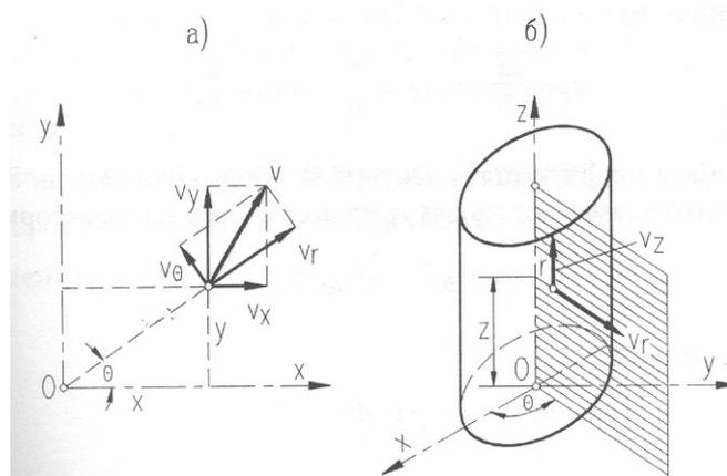
Fig. 3.3: Cartesian versus polar (cylindrical) system and axisymmetric flow
