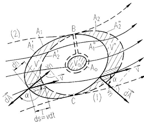
Fig. 4.16: Flow through an arbitrary finite control volume
