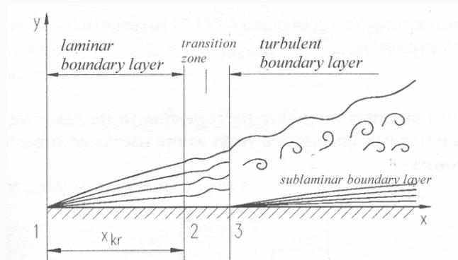
Fig. 6.11: Laminar and turbulent boundary layer
