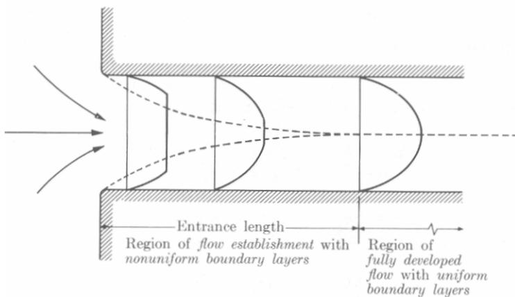
Fig. 6.10 c: Boundary layers in ducts
