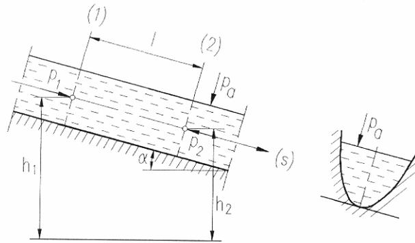
Fig. 8.6: Open channel - hydraulic gradient
