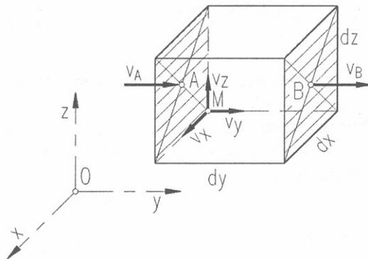
Fig. 3.16: Flow through a prismatic element
