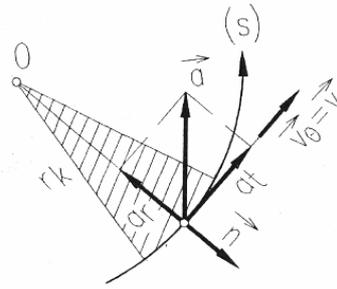
Fig. 3.18: Acceleration components in polar coordinates
