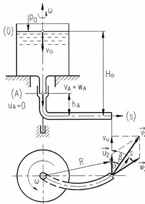
Fig. 5.16: Flow through a rotating pipe
