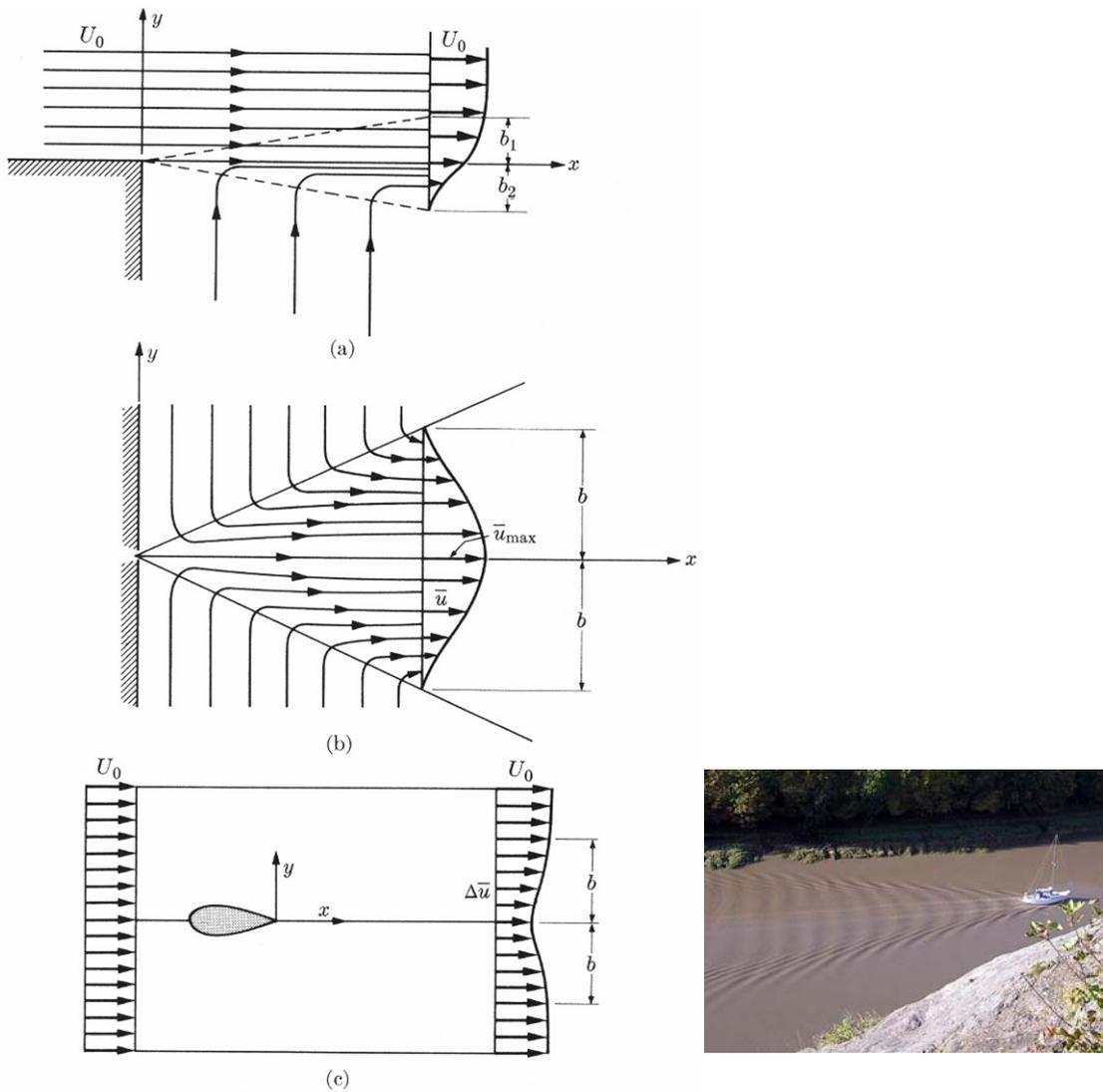
Free turbulent flows: (a) spreading at the edge of a plane jet; (b) velocity distribution developed immersed jet; (c) velocity distribution in the wake of an immersed object.
