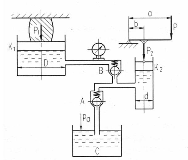
Fig. 2.11: Illustration of a hydraulic press
