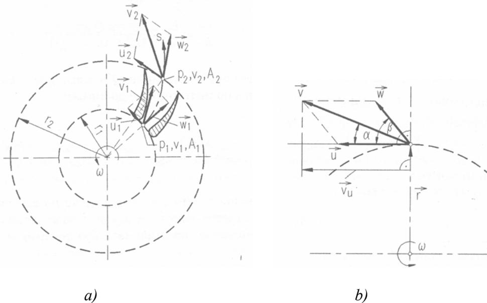
Fig. 5.27: Rotating channel of a turbomachine
