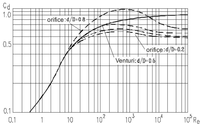
Fig. 7.2: Discharge coefficient for orifice meter and Venturi meter in function of  $Re$
