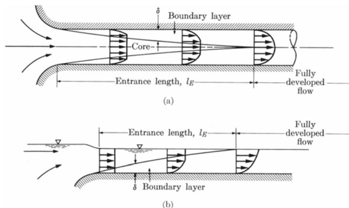
Fig. 8.3A: Developmet of uniform boudary layers: a) circular tube; b) 2-D open channel
