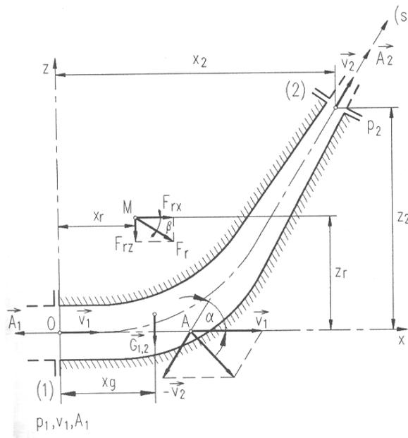
Fig. 5.24: Force on a bended pipe
