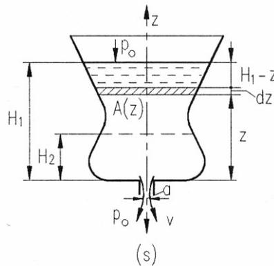
Fig. 5.15: Emptying of a reservoir
