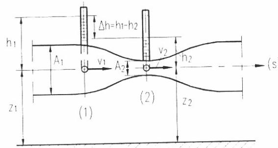
Fig. 5.5: Concept of Ventury tube (Ventury meter)
