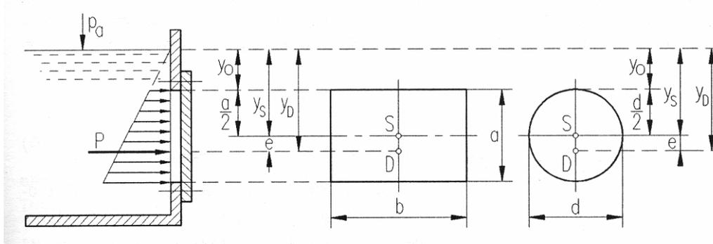
Fig. 2.15: Example - pressure force on a flat surface
