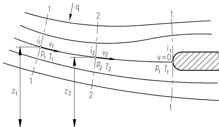
Fig. 4.20: First Law of thermodynamics - properties of fluid flow
