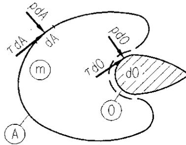
Fig. 4.19: Forces acting on fluid mass  $m$  and possible solid body
