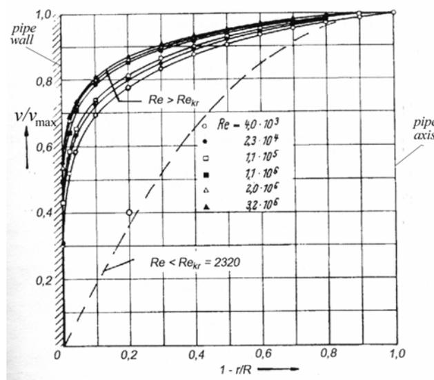
Fig. 8.10: Velocity profiles in pipe according Nikuradze
