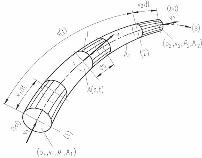
Fig. 5.1: Main properties of a stream tube
