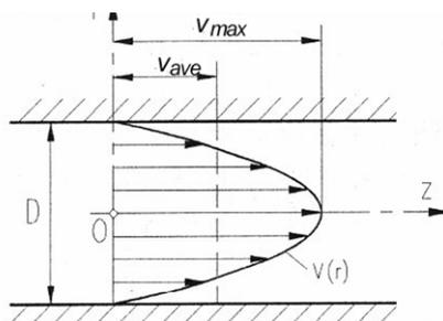
Fig. 8-8: Steady laminar flow in a circular tube of a constant diameter
