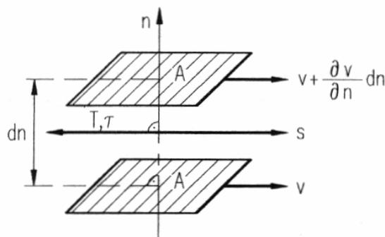
Fig. 1.1: Laminar shear of fluid between two plates
