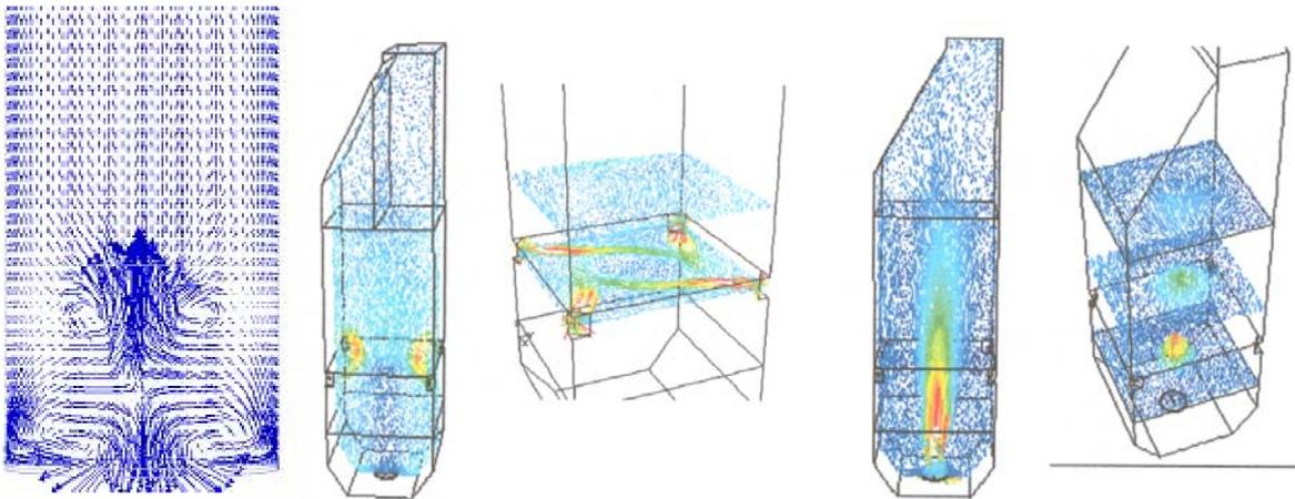
Flow field of a process in a fluidised bed
