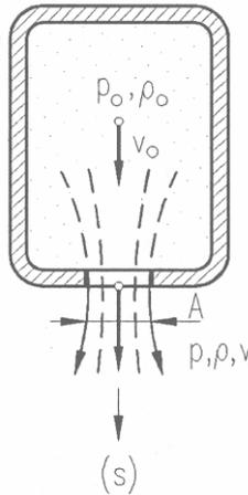
Fig. 5.22: Discharge of compressible fluid
