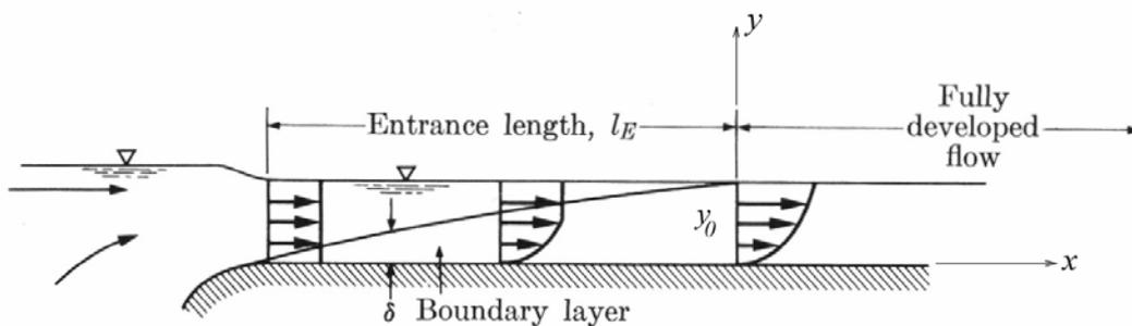
Fig. 8.18: Velocity profile for steady uniform 2-D flow in open channel
