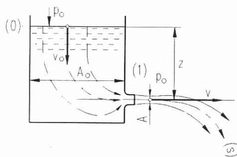
Fig. 5.7: Discharge through a small nozzle
