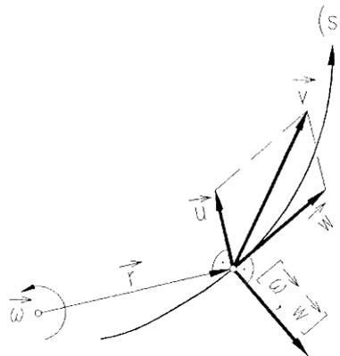
Fig 4.4: Flow along a rotating streamline
