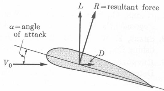
Fig. 6.13: Lift and drag on a hydrofoil section
