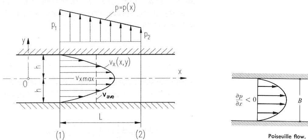
Fig. 8.14: Two dimensional flow between two plates
