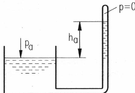
Fig. 2.9: Barometer Principle
