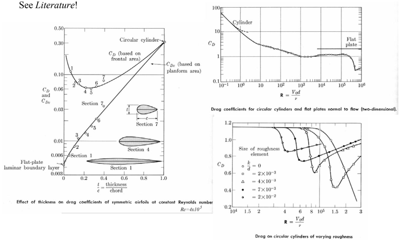
Fig. 8.19: Some data for the drag coefficients for symmetric bodies
