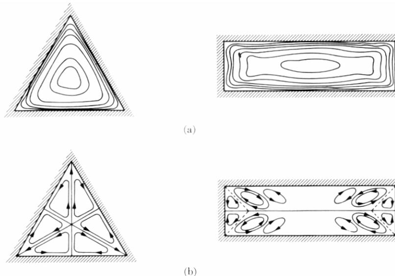
Fig. 8.12: Velocity contours and diagrams of secondary motions for fully developed flow in noncircular ducts: (a) velocity contours; (b) secondary circulation patterns [2].
