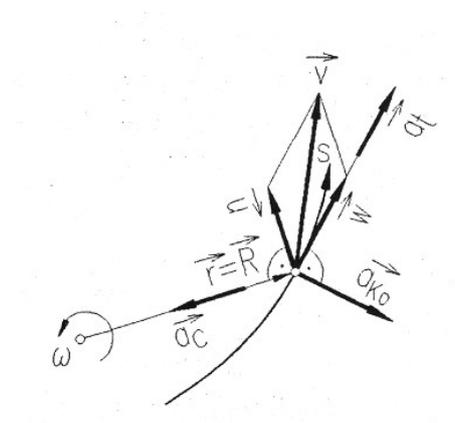
Fig. 3-20: Velocity and acceleration components of flow along a rotating streamline
