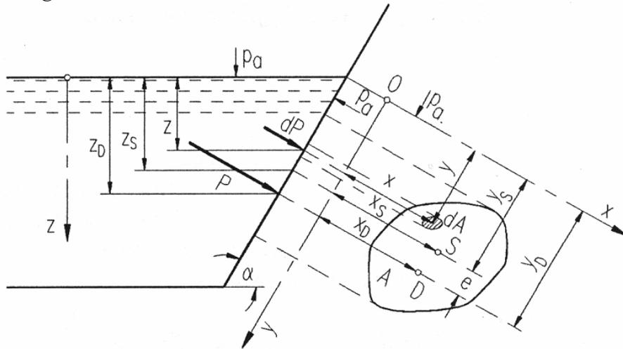
Fig. 2.14: Pressure force on a flat surface
