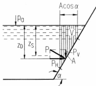
Fig. 2.16: Horizontal and vertical components of a pressure force
