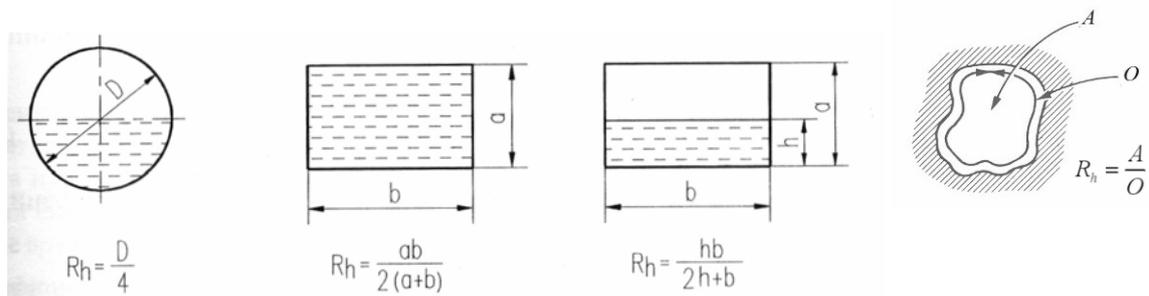
Fig. 8.5: Conduit cross-sections and hydraulic radius
