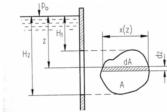
Fig. 5.10: Discharge into the atmosphere through large opening
