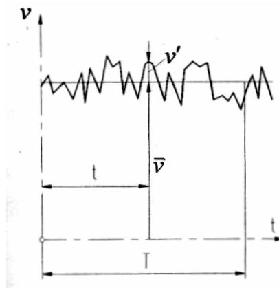
Fig. 6.17: Turbulent flow instantaneous velocity
