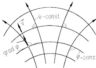
Fig 4.5: Stream lines versus equipotential lines
