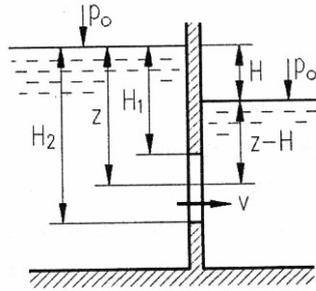
Fig. 5.12: Submerged discharge
