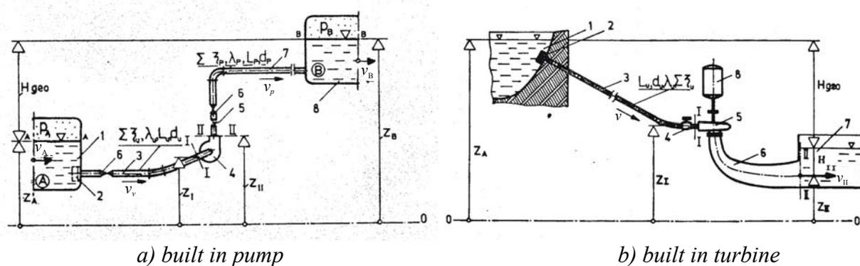
Fig. 8.7: Schemes of pipelines with built in hydraulic machine
