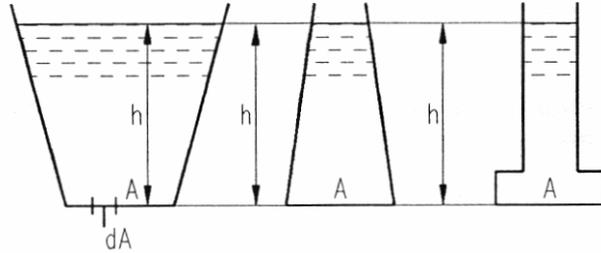
Fig. 2.17: Pressure force on horizontal bottom
