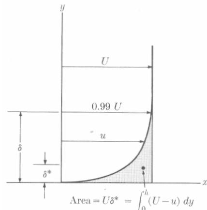
Fig. 6.10 d: Boundary layer thickness
