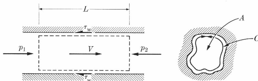
Fig. 8.13: Free-body diagram for steady flow in a constant-area conduit.
