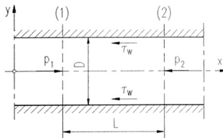
Fig. 8.4: Shear stress at pipe wall
