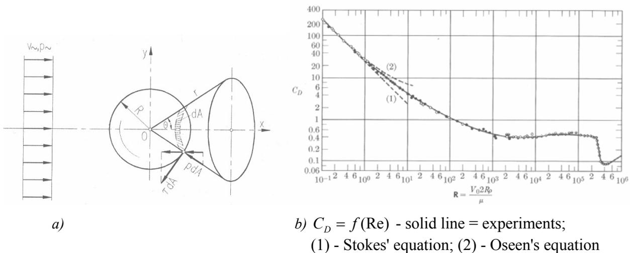
Fig. 6.9: *Creeping flow around a sphere*
