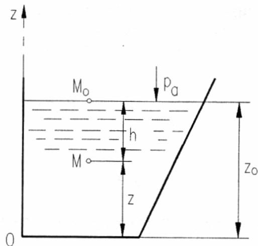
Fig. 2.6: Liquid with free surface in gravity field
