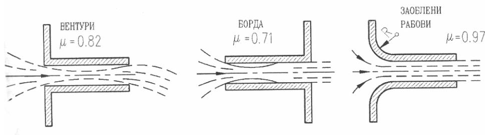
Fig. 5.9: Discharge coefficient for some nozzles
