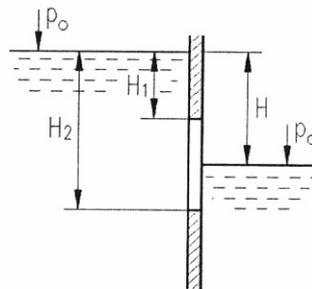
Fig. 5.13: Partially submerged discharge
