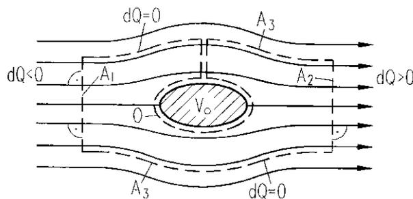
Fig. 4.18: Usual definition of a control surface
