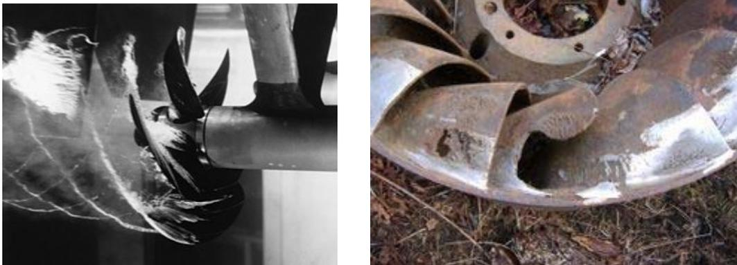
Fig. 5.17a: Cavitation generation in a propeller (a) and cavitation damage of a turbine (b).
